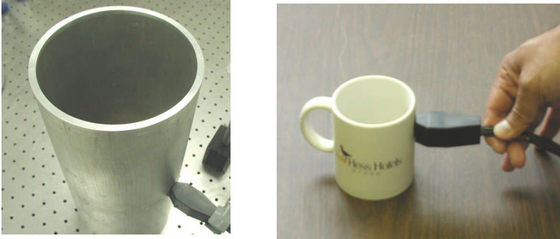
Figure 1. Simultaneous measurement of sound speed and wall thickness of any container or pipe. (a) Measurement on an aluminum pipe is shown. (b) shows measurements being made on coffee mug for which there is no available sound speed data. The black sensor head needs to be in physical contact with the object as shown above.
